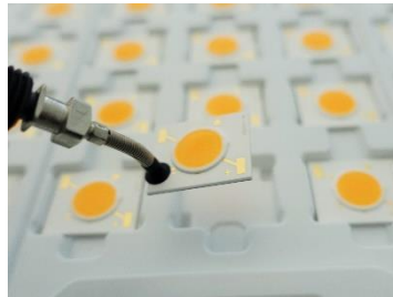
Figure 9. Removing the COB LEDs from the Tray with Vacuum Tweezers
