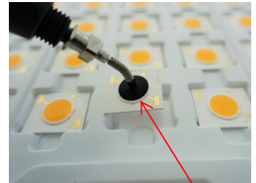
Figure 9. Removing the COB LEDs from the Tray with Vacuum Tweezers
