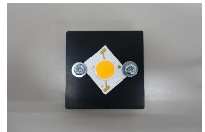
Figure 16. Do Not Attach the COB LEDs with Screws
