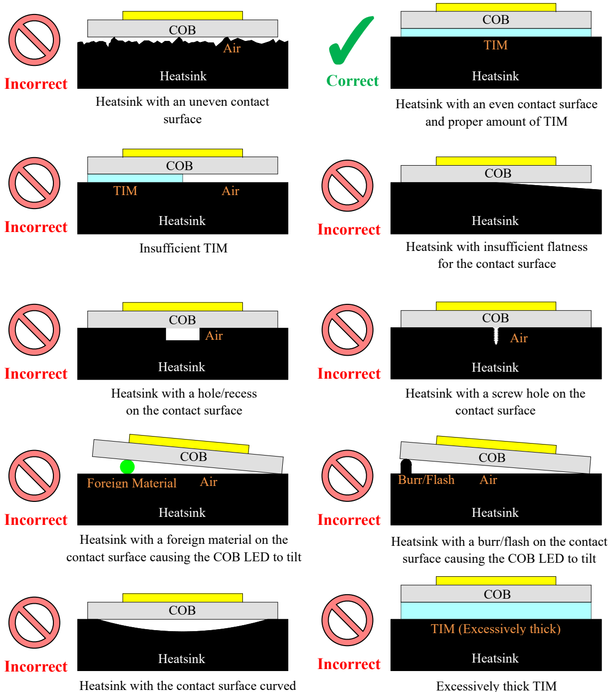
Figure 11. Correct/Incorrect Examples of Attaching a COB LED to a Heatsink
